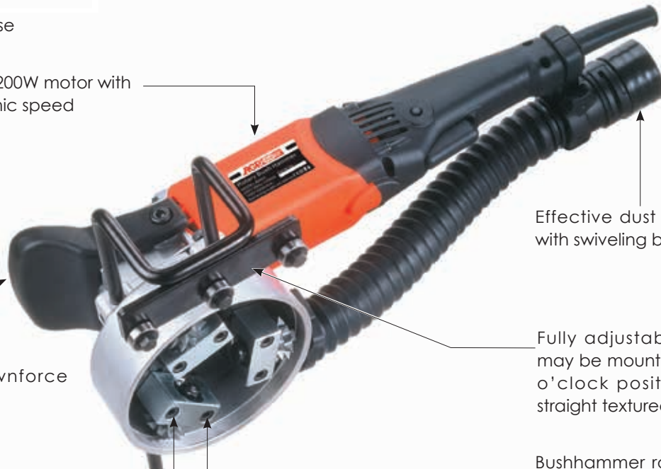
Bushhammer rolls (included) can be mounted to create 51, 70, 96, or 116mm wide textured strips
